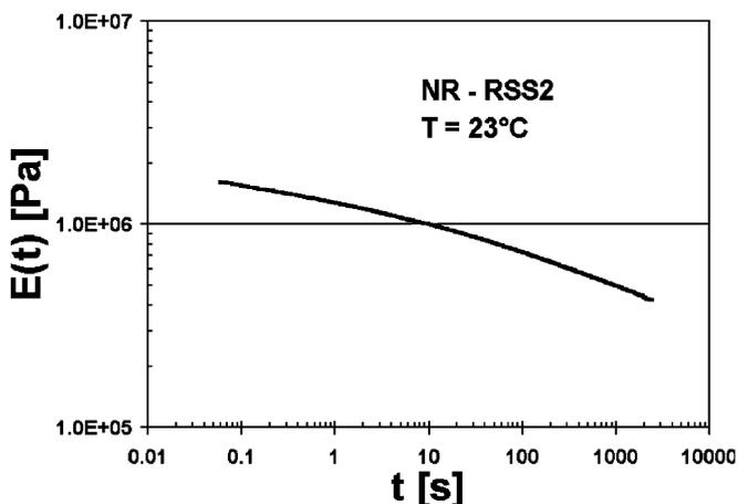
**Fig. 7** Extensional stress relaxation modulus for NR-RSS2 for a step Hencky strain of 0.2 at 23 °C
