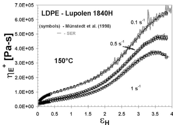
**Fig. 6** Comparison of the tensile stress growth function versus Hencky strain curves obtained with the SER (solid gray lines) and data from the literature (black symbols from Münstedt et al. [20]) for the same low-density polyethylene (LDPE) (BASF Lupolen 1840H) at a melt temperature of 150 °C and for Hencky strain rates of 0.1 s<sup>-1</sup>, 0.5 s<sup>-1</sup>, and 1 s<sup>-1</sup>
