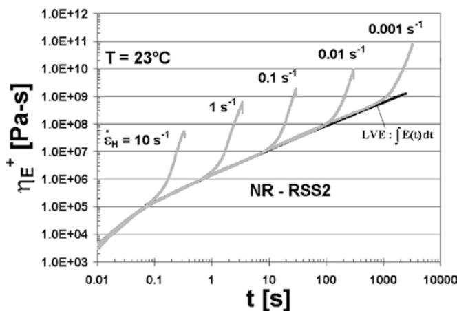
**Fig. 8** Tensile stress growth curves for NR-RSS2 for constant Hencky strain rates ranging from 0.001 to 10 s<sup>-1</sup>
