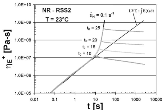
**Fig. 9** Cessation of steady extension curves for NR-RSS2 at 23 °C for a steady Hencky strain rate of 0.1 s<sup>-1</sup> stopped at a test time,  $t_0$ , of 10, 15, 20, and 25 s. Note the excellent reproducibility of the growth curves. LVE Linear viscoelastic
