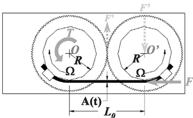
**Fig. 2** Force diagram indicating the tangential stretching force,  $F$ , on the slave drum and the resultant torque,  $T$ , measured by the torque transducer of a de-coupled drive motor and torque transducer host system.  $\Omega$  Drive shaft rotation rate,  $R$  radius,  $A(t)$  instantaneous cross-sectional area,  $O$  sum of moments about the drum's axis of rotation,  $F$  tangential force
