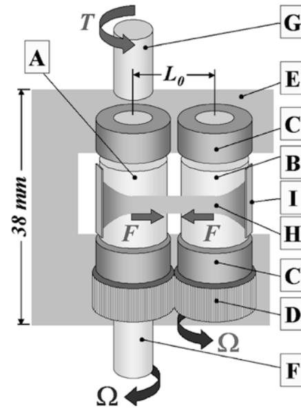
**Fig. 1** Schematic view of the Sentmanat extensional rheometer (SER) during operation. Inside squares: A Master drum, B slave drum, C bearings, D intermeshing gears, E chassis, F drive shaft, G torque shaft, H sample, I securing clamps. Other symbols:  $L_0$  unsupported length,  $\Omega$  drive shaft rotation rate,  $T$  torque,  $F$  tangential force
