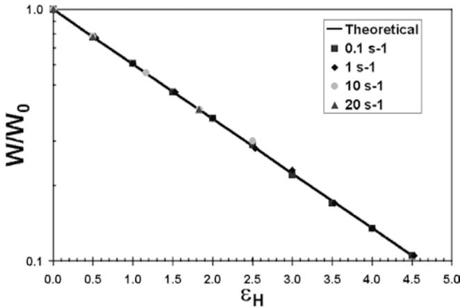
**Fig. 4** Strain validation plot for the SER-HV-A01 Universal Testing Platform measured with a multitude of materials at Hencky strain rates up to  $20 \text{ s}^{-1}$
