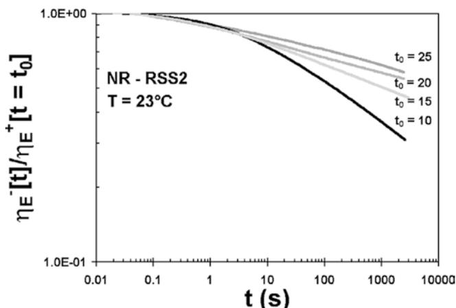
**Fig. 10** Relative stress relaxation curves for NR-RSS2 at 23 °C from cessation of steady extension experiments demonstrating the effect of strain-induced crystallization behavior on stress relaxation
