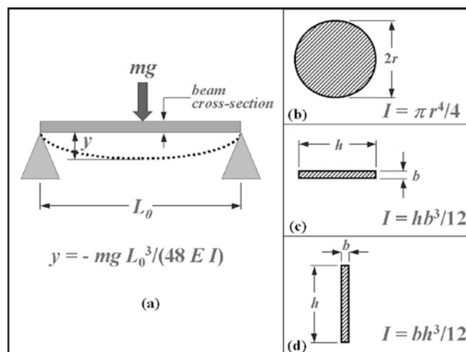
**Fig. 18a–d** Simply supported beam deflection diagram for a mid-span beam weight concentration (a) and the corresponding flexural moment of inertia,  $I$ , depicted for three types of beam cross section: b circular beam section, c flat rectangular beam section, and d upright rectangular beam section
