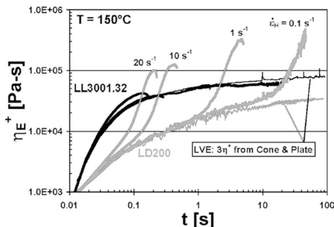
**Fig. 15** Tensile stress growth curves for LD200 and LL3001.32 at 150 °C superposed with the LVE  $3\eta^+(t)$  shear stress growth curves for each polymer taken from cone and plate measurements in start-up of steady shear at 150 °C
